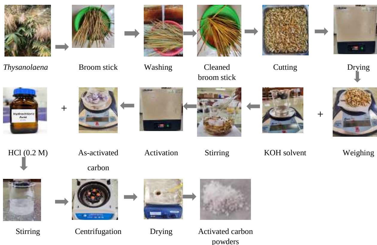
Figure 1 Synthesis process of activated biochar powders by one-step chemical activation process
